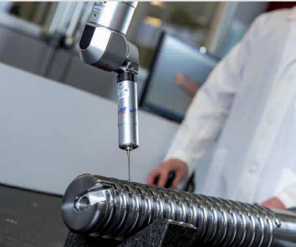
ZEISS ACCURA Bridge Type Measuring machine; measuring range 1200x1800x1000 mm Portal Messgeräte; Messbereich 1200x1800x1000 mm
